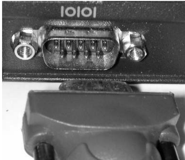
Figure 1.8 Null Modem Cable Attached to a Laptop
