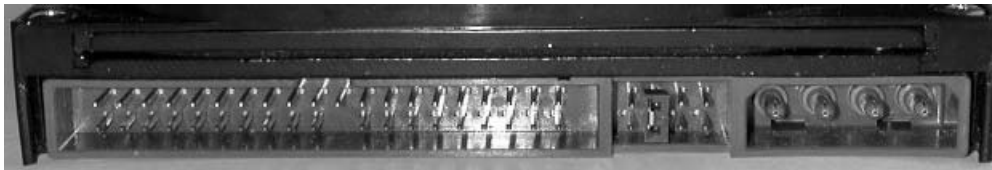
Figure 13.1 IDE Hard Drive Connectors
