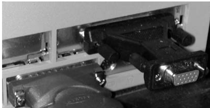
Figure 1.7 Null Modem Cable Attached to a SPARC System
